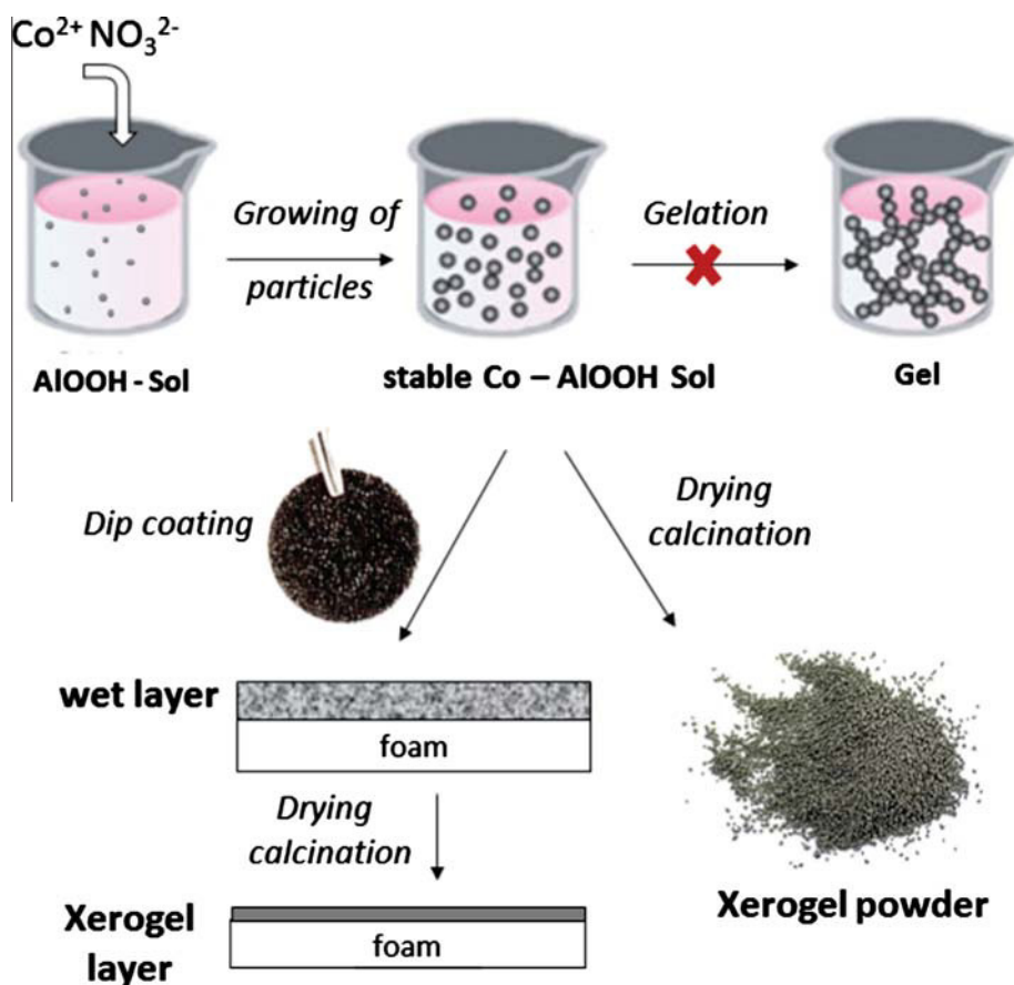
Fig. 1. Preparation route of xerogel powders and xerogel coated foams.
